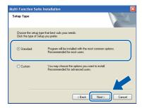
When this screen appears, connect the USB interface cable to your PC, and then connect it to the machine.
